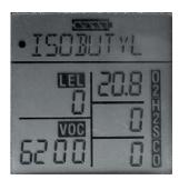
spell out the user-selected VOC of choice in the dashboard display area. The unit automatically calculates the response factor by scrolling through a "favorite-five" list or by selecting a gas from a 100-gas pre-programmed list. Customized chemical names and corresponding response factors can also be easily added to this list. A userselectable option to enable ppb VOC readings below 10 ppm provides additional flexibility.
